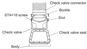
The exhaust wall hole diameter shall be close to that of the exhaust pipe, which shall not be too small. Otherwise, it will cause poor exhaust efficiency, more noises and lower airflow, etc. The connection between the pipe and the hole or the public flue must be sealed tightly to ensure that, the pipe and the check valve or public flue are connected securely. The blades at the check valve connection or public flue connection must be flexible.
