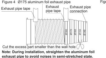
Excess part may be cut with a wire cutter.
